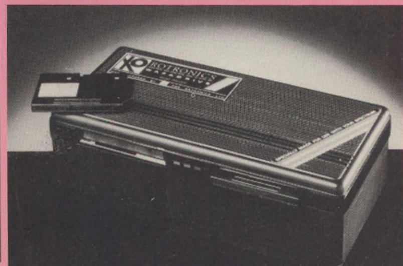
Rotronics Wafadrive – mass storage and printer ports.
